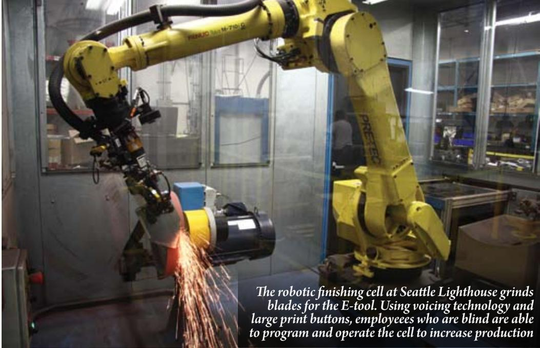
*The robotic finishing cell at Seattle Lighthouse grinds blades for the E-tool. Using voicing technology and large print buttons, employees who are blind are able to program and operate the cell to increase production*
